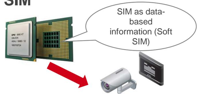
A communication module given SIM functions where the information required for mobile communications is logically written in internal memory
