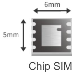
Embedded Chip-type SIM (M2M UICC)
