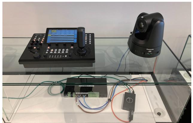
Photo 10: Panasonic PTZ Remote Controller and Remote Camera
