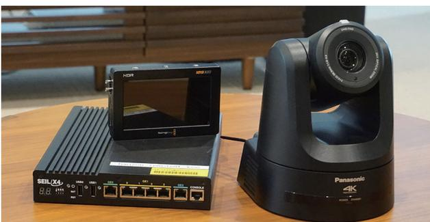
Photo 12: SEIL Router Used to Build L3VPN (left) and PTZ Remote Camera (right)
