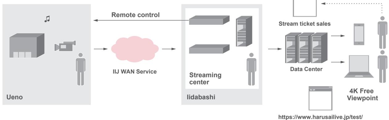
Figure 1: Live-Streaming System Configuration Comparison (2021 & 2022)
