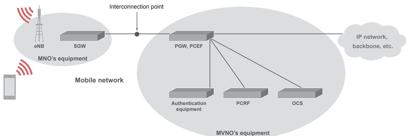
Figure 10: Connection Sequence from Mobile Phone to MVNO Network
