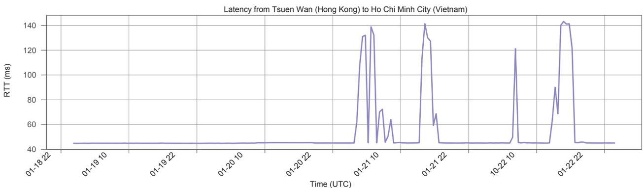
Figure 12: Latency between Hong Kong and Vietnam during Asia-America Gateway (AAG) cable reconfiguration (January 2018)
