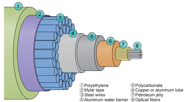
Figure 2: Cross Section of Submarine Cable with Multilayer Protection
