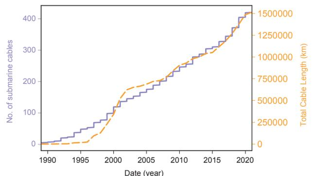
Figure 4: Number of Cables and Total Cable Length
