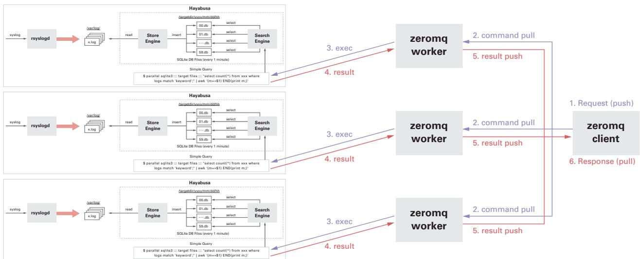
Figure 5: ZeroMQ Push/Pull Implementation Used With UDP Hayabusa
