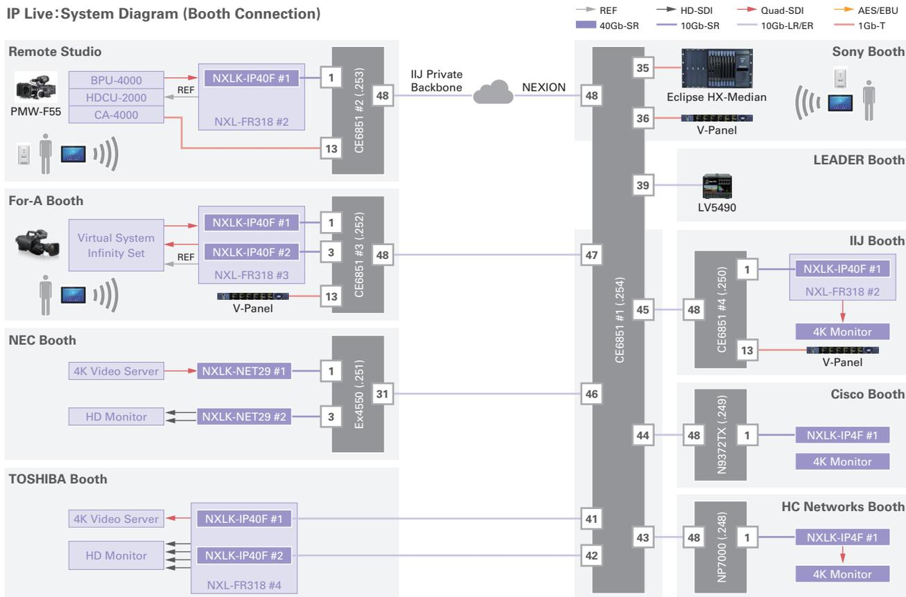
**Figure 4: Remote Production Example at Inter BEE 2017**
