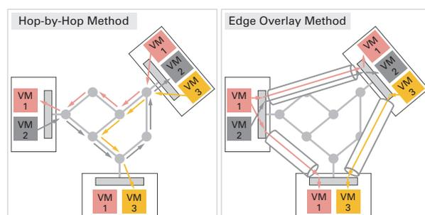
Figure 2: Hop-by-Hop Method and Edge Overlay Method
