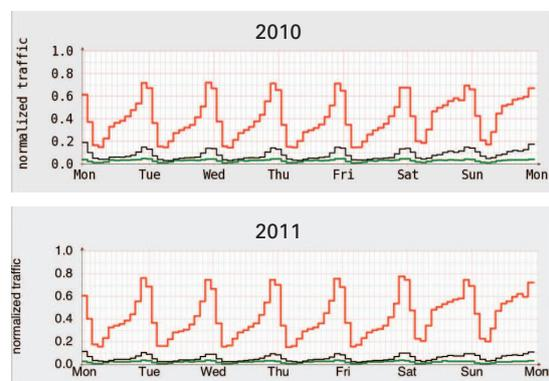
Figure 7: Weekly TCP Port Usage Trends for Client-Type
